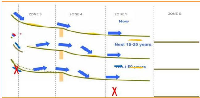
Figure 7: Schema of Sediment Loss in Flow to Mekong Delta down-stream. Thus, the current tendency is to significantly reduce the movement of fine alluvium, due to the operation of large reservoirs in China and its tributaries. In the 20-year future scenario, the sediment load in Zone 2 will be reduced by 80%, while down-stream in Kratie (Cambodia) this amount will be halved. The estimated alluvium is 90 million tons /year in Chiang Saen (Chang Rai); Amount of 84 million tons /year in Vientiane plus an additional 25 million tons /year in Se San, Sekong, Srepok and 56 million tons /year from the basin between South Binboun and Se Done, totaling about 165 million tons coming in Kratie. With hydro-power on tributaries and up-stream basin, these amounts will be reduced by about 20 million tons /year (in Chiang Saen and Vientiane), 88 million tons /year (in Kratie). With the tendency of 2030 without more main-stream dams, the sediment load will be halved to be smooth and nutritious to the Mekong Delta (Table 5).
